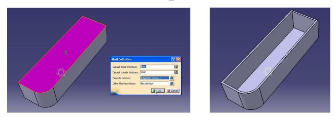
If you want to create wall thickness to the outside, enter the Default outside thickness value. You can also create wall thickness in booth directions.
